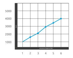
The Normal liter/hour air consuption depends on applid pressure, users number and point connection tube diameter (be careful in case of spray, nozzle diameter must be kept into account).
