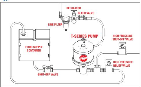
NOTE: T-Series Pump is the only item supplied by HiP with order of pump. All other components are available from HiP to be ordered separately.
