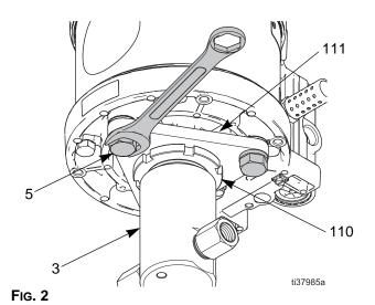
5. Slide the pump lower (3) off of the pump, with the lower bracket (111) and locking ring (110) still attached to the pump lower.
