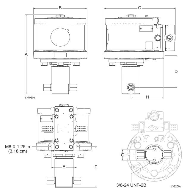
Fig. 12 T-Series Pump Dimensions and Mounting Holes
