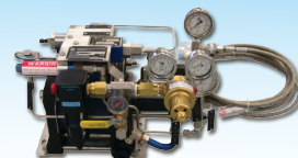
Portable Booster System with Safety Valves
